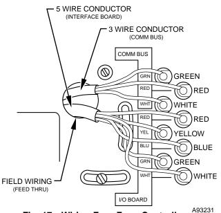
Fig. 17—Wiring Four Zone Controller
